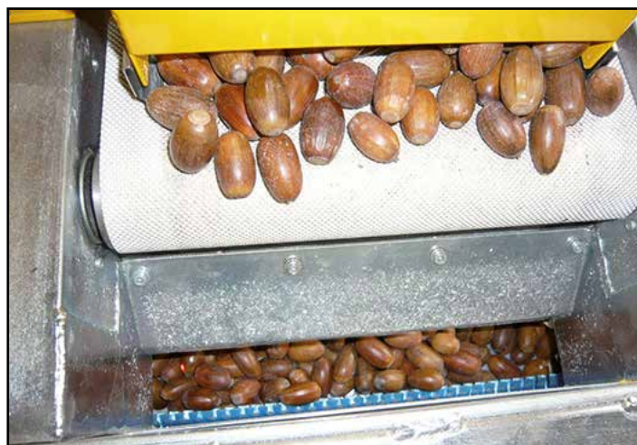
belt conveyor for feeding Acorns to the distribution box
