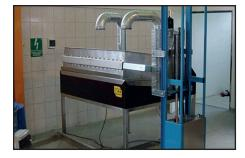
The wet seedlot is placed in a dryer box with perforated bottom to allow for air flow through the seedlot to allow it to dry faster. A high volume air stream blows through the seed to dry the seed for the next process.
