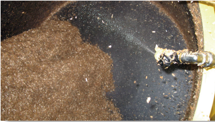
dewinging by the means of spraying water
