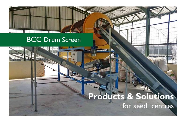
The BCC Drum Screen is a versatile and multi-functional piece of equipment used for various purposes in forest seed processing plants and containerised nurseries. Some of the uses include pre-cleaning of cones/pods/capsules, large scale extraction of seed, screening of growing media for nursery use, and pre-cleaning of inserts before washing and sterilizing.
