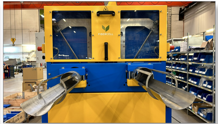
2 pipes with cell diameter from 90 to 120 mm
