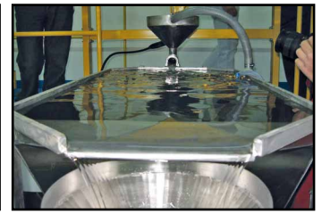
seed is transferred continuously by the tank overflow stream
