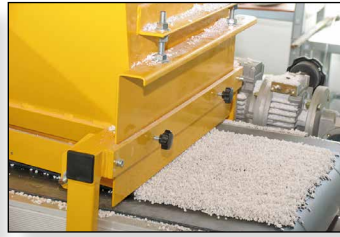
adjustable gate to determine thickness
