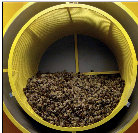
insert drum is filled with cones for seed extraction
